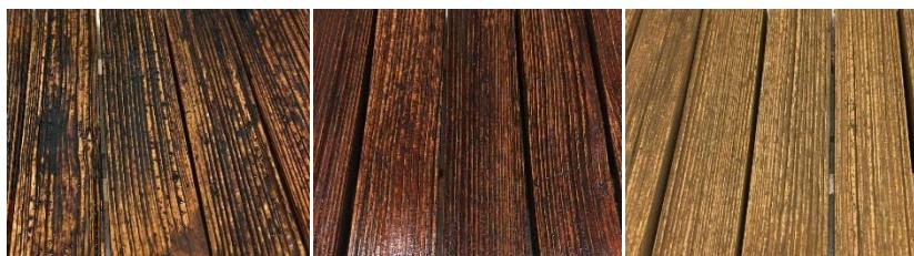
Figure 1 Different types of used coatings, from the left – Wood Tar, Carbolineum EXTRA and Luxol
