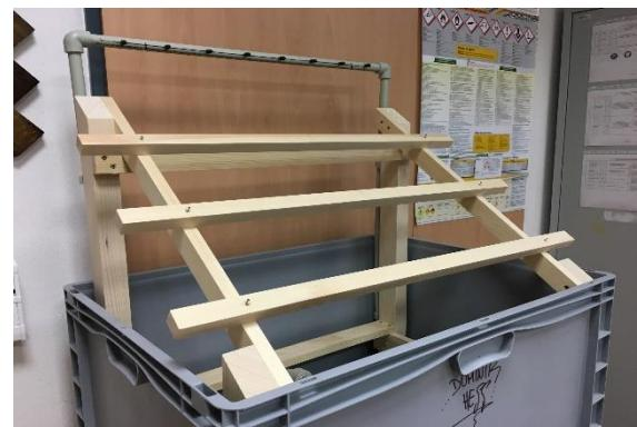
Figure 2 Wooden construction made for artificial rain.
