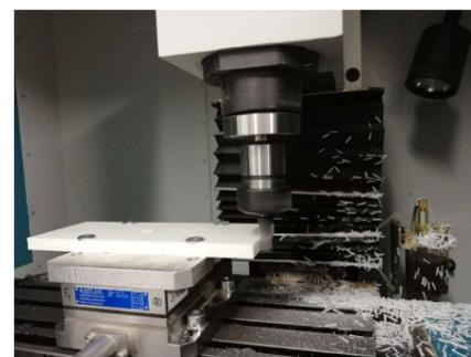
Fig. 3 Milling of artificial stone Corian
