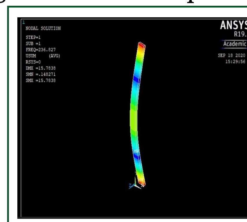
Fig.1. First bending mode of the beech wood made by ANSYS R19.2. The referred frequency value is 236.8 Hz, (material model from Hearmon, 1948)
