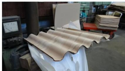
Fig. 3 Corrugated plywood panel
