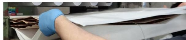
Fig. 5 Silicone and wax paper was inserted in two layers from each side
