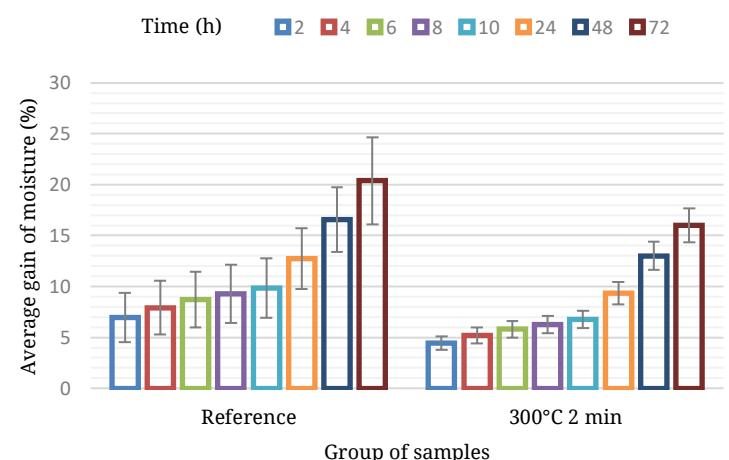
**Figure 3:** Tangential moisture measurement. The best optimization for carbonization of tangential samples was 300°C 2 min.
