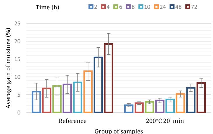
**Figure 4:** Radial moisture measurement. The best optimization for carbonization of radial samples was 200°C 20 min.
