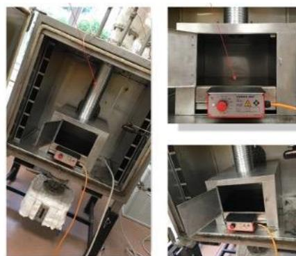
**Figure 1:** Contact heating laboratory device with built-in NiCrNi sensor and electronic controller with range 50 – 500 °C.
