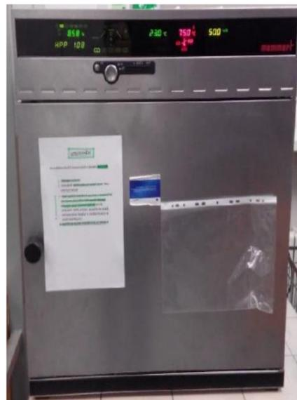
Figure 3 Memmert HPP 108 - climatic chamber
