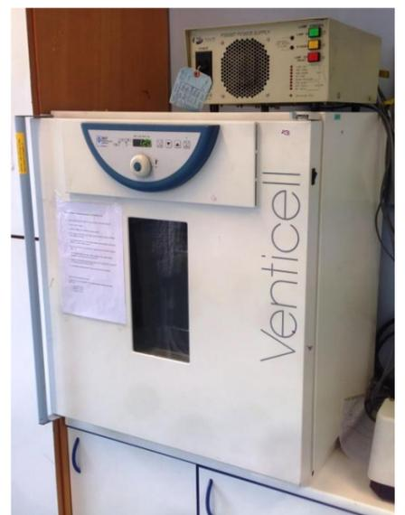
Figure 4 VENTICELL 111 - hot air dryer
