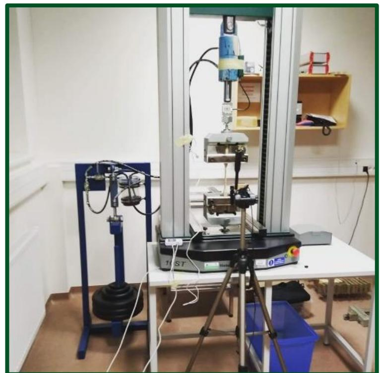
Figure 1 Creep testing kit
