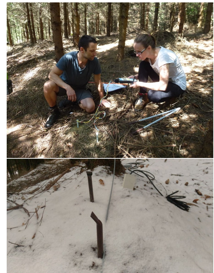
Figure 1: Field measurement with Z meter (up); blinding plugs in the holes for probes (bottom).
